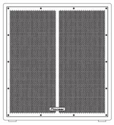
The XY-118S is a compact, powerful subwoofer product designed for a wide variety of sound reinforcement applications where power and LF extension are required within a compact footprint. It features a high-power 18 inch (457 mm) ferrite LF drive unit in an optimally tuned reflex enclosure, resulting in a response which has incredible depth for an enclosure this size, yet still retains speed and impact.
