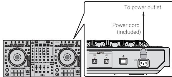
6 Press the [POWER] switch on this unit's rear panel to turn this unit's power on.
