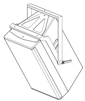
Ensure that both the flat and locking washers are used – the flat washer should be in contact with the cradle. Tighten the bolts to ensure a solid fit. Once the desired angle of the loudspeaker is set, tighten the levers on the cradle to lock the position in place. The points on the top of the flying cradle can be used for permanent installations or to secure a hook clamp.
