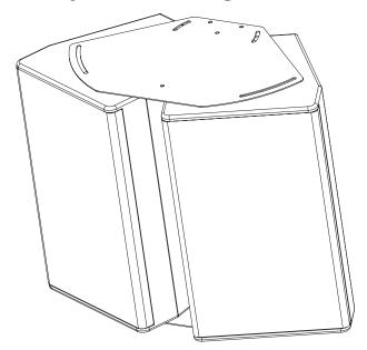
Using the supplied M10 socket head bolts, bolt through the CP-XY15DF1 plate into the enclosures. Ensure that both the flat and spring washers are used — the flat washer should be in contact with the plate. Once the desired angles of the loud-speakers are set, tighten the bolts to lock in place. Then turn the cluster over and repeat the process on the bottom. Use the top points on the XY-152 enclosures as a secondary safety feature.
