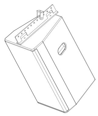
Using the supplied M10 hex head bolts, align the mounting holes in the flying bracket with the mounting points on the top or the bottom of the enclosure. Ensure that both the flat and locking washers are used — the flat washer should be in contact with the cradle. Tighten the bolts to ensure a solid fit. Finally, attach a hook-clamp to the mounting point.
